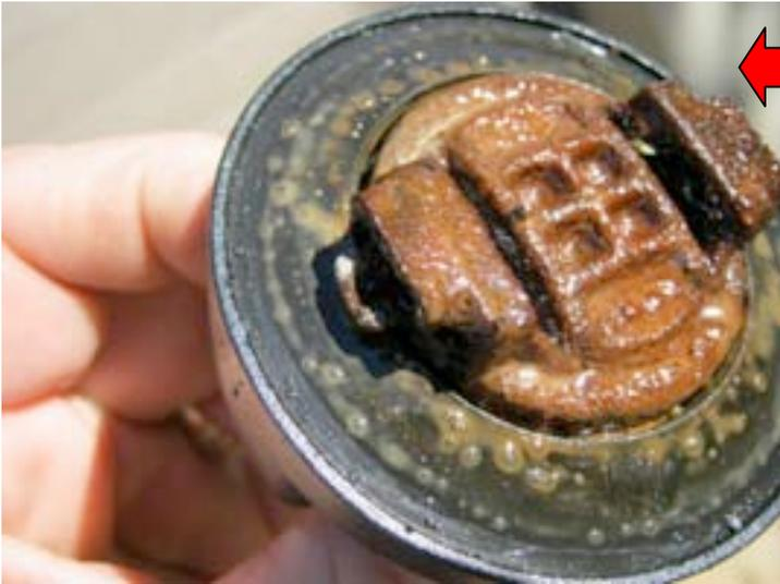
This vehicle was used only locally, and rarely at full operating temperature. A strong build up of sludge, with water droplets from condensation is evident. The vehicle was a 2008 model.
