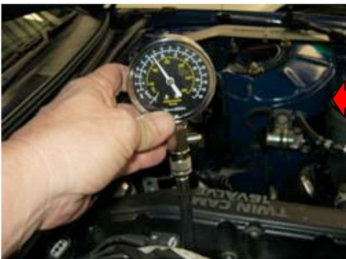
Make sure the engine is sound from inside. Have a compression check.
