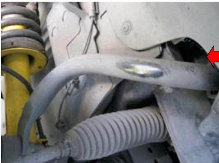
This vehicle had oversized tyres fitted which interfered with the operation of the suspension, causing early tyre and structural wear.
