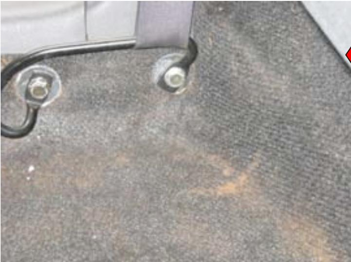
This carpet in the back passenger floor of this Toyota is starting to show signs of staining, misshape and shrinkage. In addition, the seat belt retaining bolts exhibited slight corrosion, indicating possible water damage. On further investigation this car was found to be recently brought from interstate with expected flood damage.
